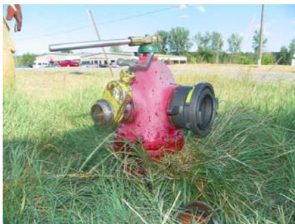
**2. Making the hydrant** - This seems like such a simple task, but can be a very dangerous one. How are you going to dress the hydrant? Are you just laying a 5-inch line from the steamer to the rig, or are you placing two 2 1/2 or 3" lines off the additional ports? Are you connecting a HUMAT valve or a hydrant assist valve on, or are you hooking directly to the hydrant? This all depends on what your SOGs are and what you are trying to accomplish. Are you using
