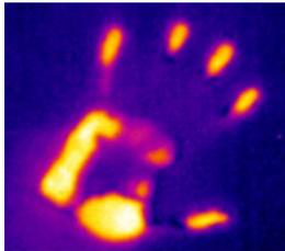
(ie) Placing your hand on a wall (non reflective) after several seconds removing your hand from the wall, view the area with a TIC and notice the light color outlining placement of your hand on the wall and its position and the difference in comparison with the rest of the wall.
